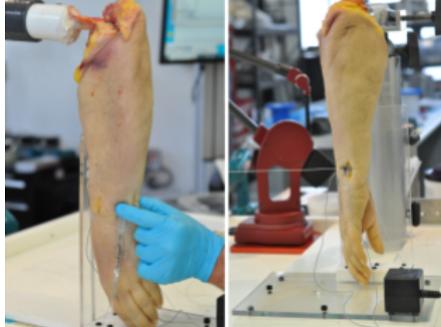
Figure 4: Overview of invasive cadaver rig for DRUJ instability quantification
